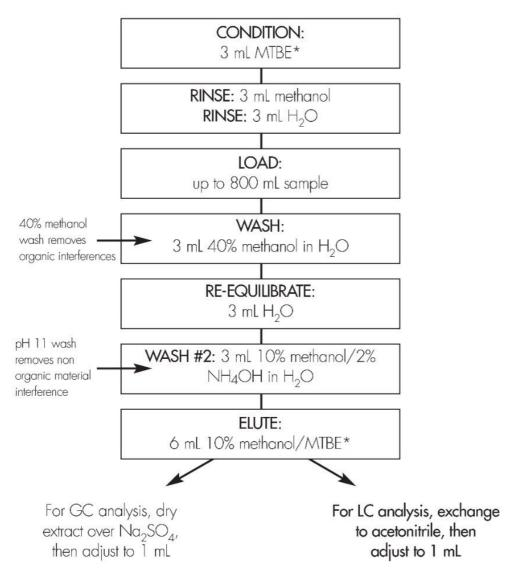
\* methyl tbutyl ether diethyl ether can be used as an alternative to MTBE
