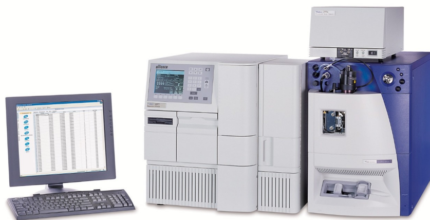
Waters Micromass Quattro micro API triple-quadrupole mass spectrometer.
