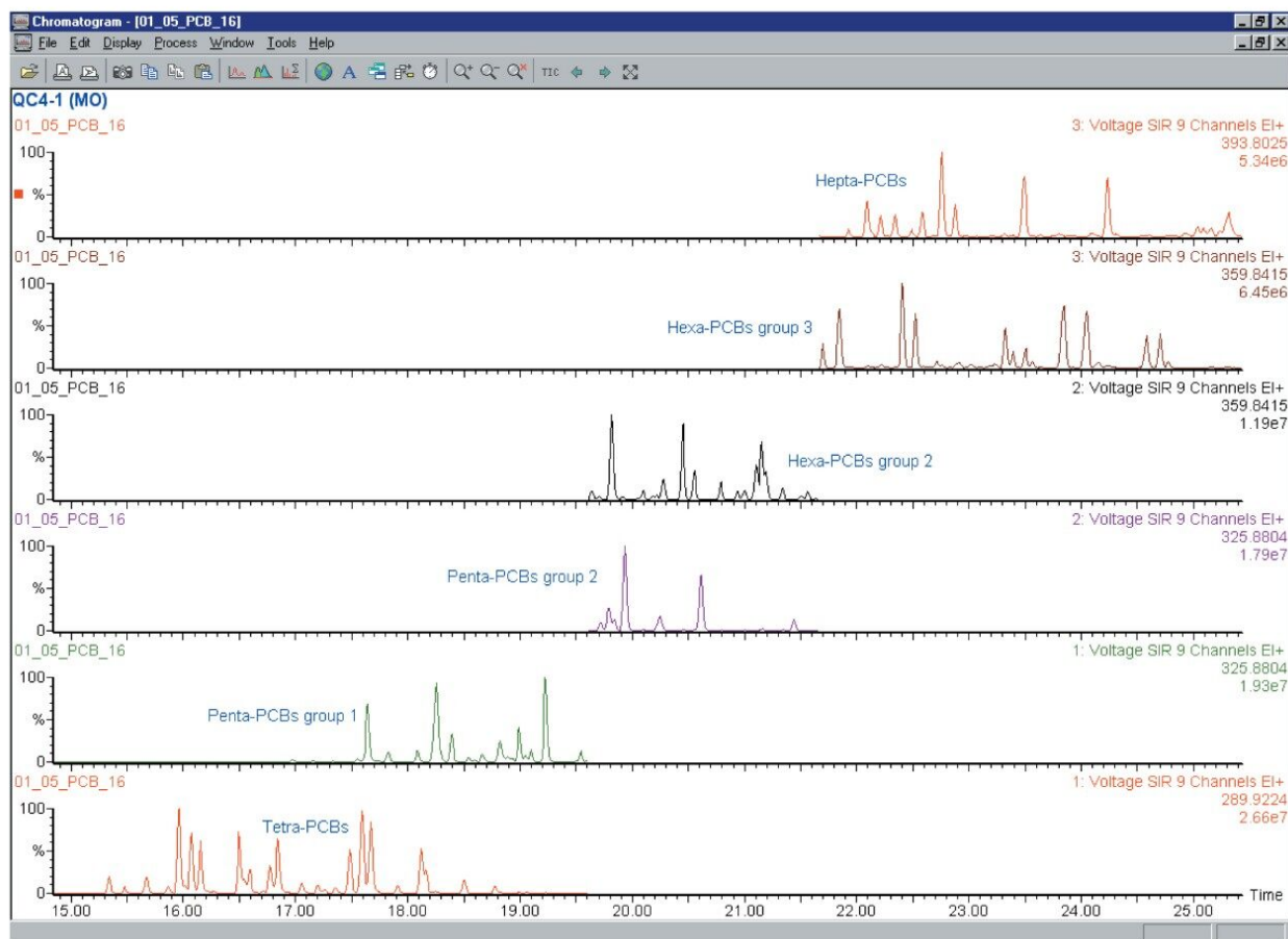
Figure 1. Typical chromatograms for WHO-PCB analysis.
