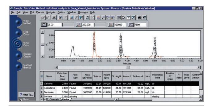
A portion of a screen capture on a Breeze System. The analysis of a diet cola shows the information that is produced together with the liquid chromatogram that the operator can examine, if desired. Note that this analysis is performed in about 6 minutes.
