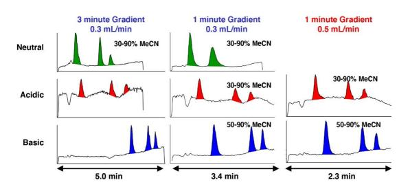
Effect of pH and Gradient on Peak Shape - overlaid extracted masses [M+H]+
