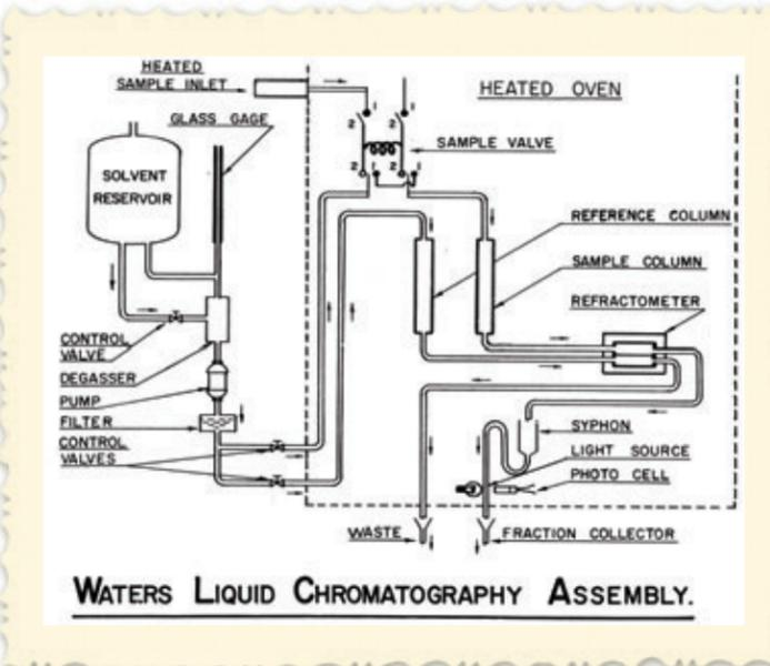
Flow schematic from page 4 of the 1963 instruction manual for the first prototype of the GPC-100. As apparent in the diagram's title, all the elements of an HPLC system were present in this instrument.
